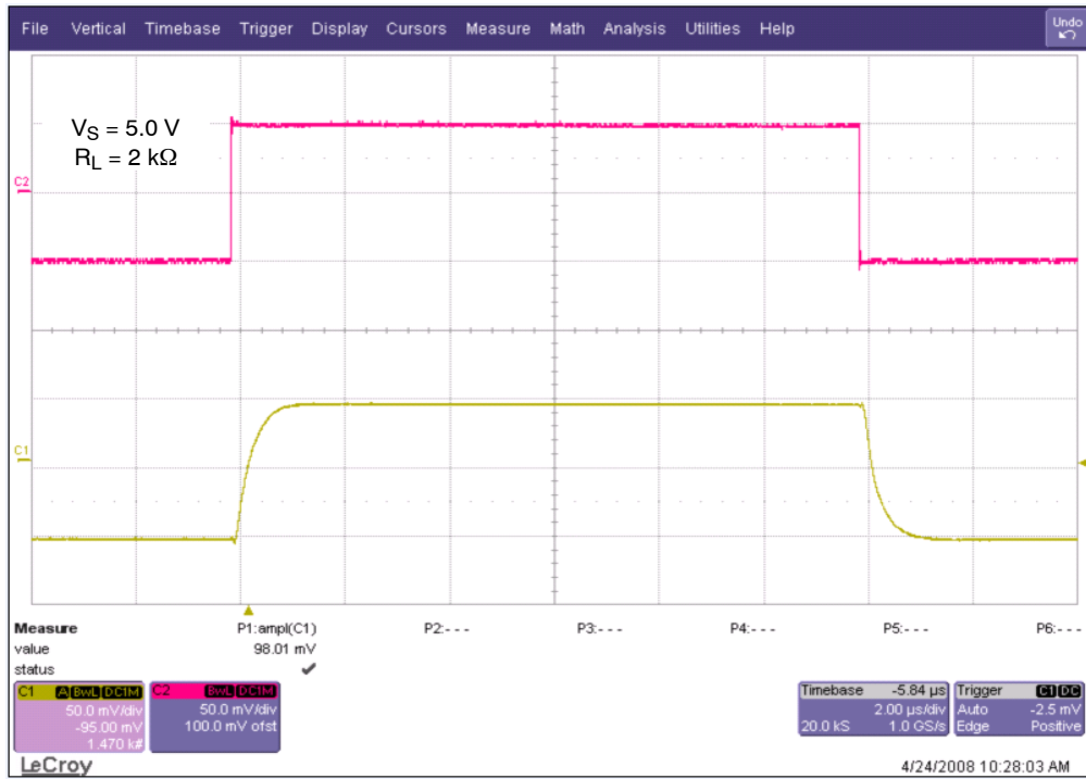
Figure 17. Small Signal Noninverting Response
