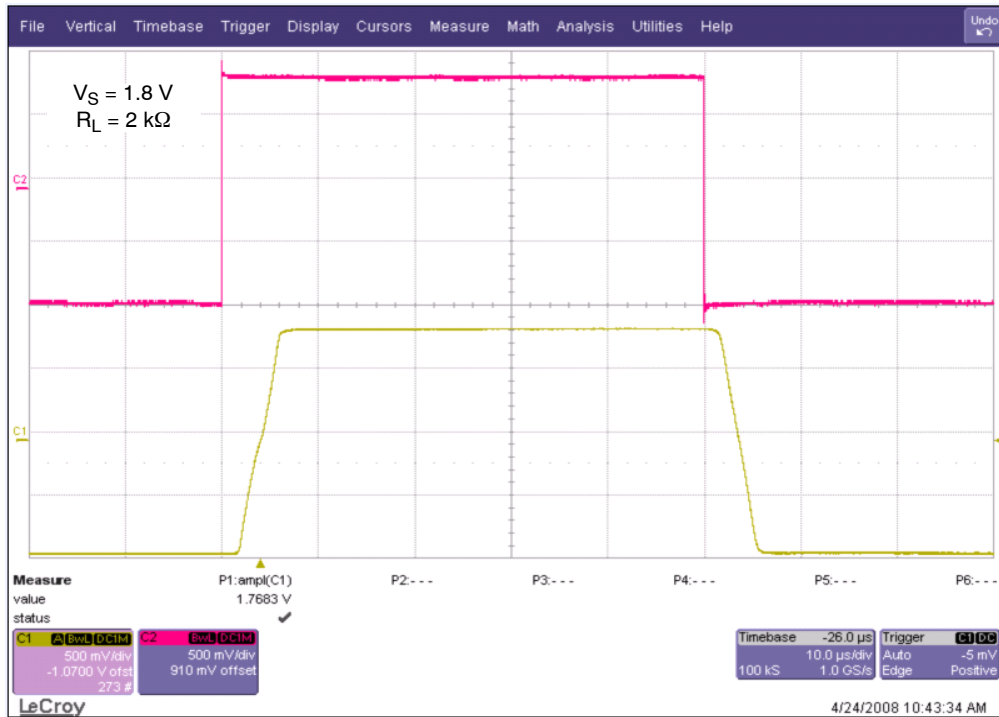
Figure 18. Large Signal Noninverting Response
